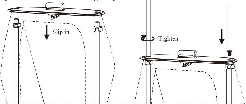
4. Install the rail on the top of the supporting aluminum rods and fix the rail with the rail screws. Lift the clothes care machine lid, put the draw hook cover on the rail and fasten the draw hook cover.
