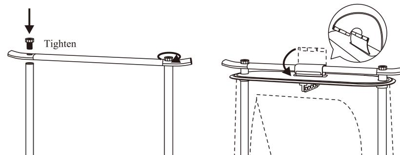
5. Adjust the hasps of the clothes tray on both sides to the right position, place the clothes tray on top, and you can place underwear or socks on the clothes tray. To meet different demands, the hasp of the clothes tray can be moved up and down to adjust height of the tray.
