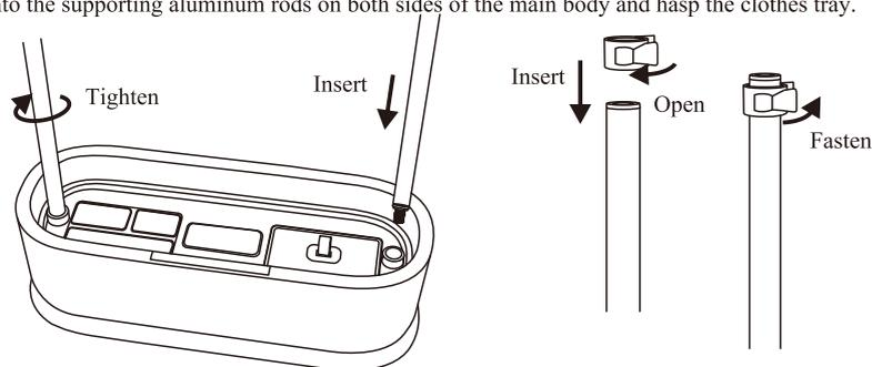
3. Slip the clothes care machine lid into the supporting aluminum rods on both sides of the main body, and then install the other two supporting aluminum rods.
